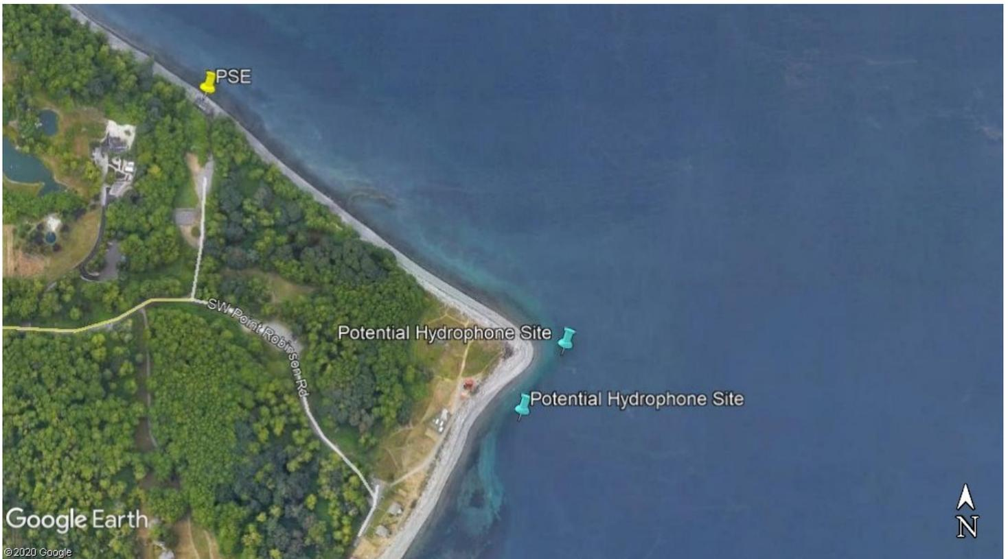
The blue markers show potential site locations for the hydrophone. Final determination would be made after acoustic testing and habitat evaluations. If the location directly off the light house is selected, the cable would run directly out from the lighthouse to the hydrophone. If the location at the point is selected, the cable could either run to the point along land line and then turn into the water, or the line could come out from the lighthouse and travel along the beach.
